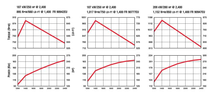
Curves shown represent gross engine performance capabilities obtained and corrected in accordance with Cummins standards. Standard conditions are: 29.36 in. Hg (99.14 kPa) barometric pressure, (500 ft [152 m] altitude, 77°F [25°C] inlet air temperature). Actual performance may vary with different ambient conditions.
